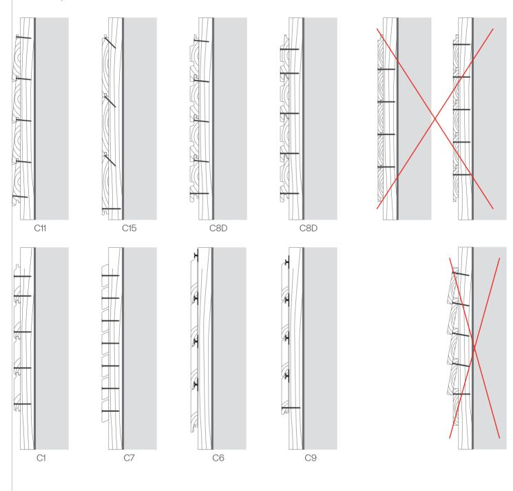
For shiplap profiles, leave an air circulation space of 2-3 mm to allow for swelling of the wooden boards. Always install shiplap cladding from the lower edge of the wall upwards.
