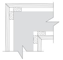
Cut the boards to a 45-degree angle.
