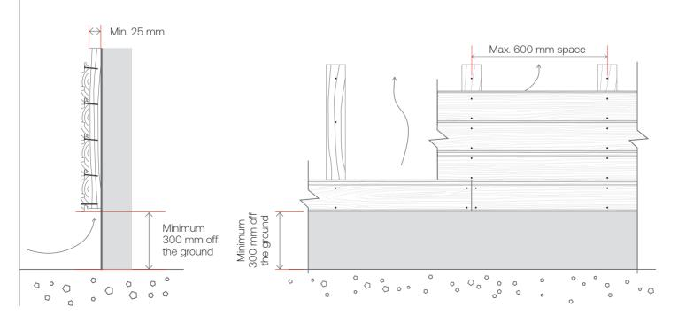
Installation guide Cladding Boards
