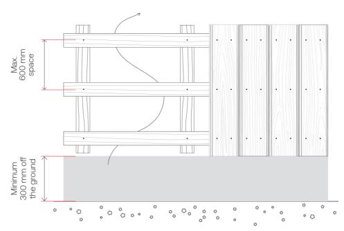
Fix **vertical cladding** onto horizontal battens; the joint ends of the boards must be resting on the battens with standard cladding boards. Joint end-matched boards can be placed with the joints meeting between the battens; this will save both material and time.
